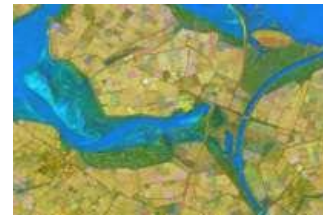
RGB composite of ERS coherence (red), average backscatter (green), and backscatter temporal variability (blue) over the Netherlands.
