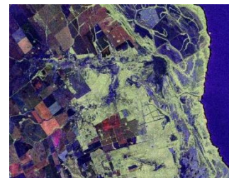
Polarimetric decomposition of quad-pol. SAOCOM L-band SLC data.
