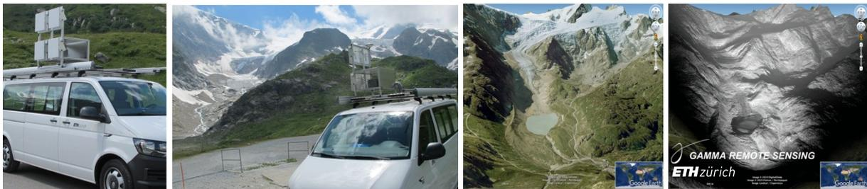
Figure 5: Left/center-left: car-borne setup of the L-band SAR system with one transmit and three receive antennas. Repeated SAR data acquisitions of the Stein Glacier were made while driving on a slightly curved section of mountain road. Center-right/right: Google Earth view of the Stein Glacier test site (CH). Geocoded intensity image (right) overlaid to Google Earth view as obtained from a car-borne L-band SAR acquisition.
