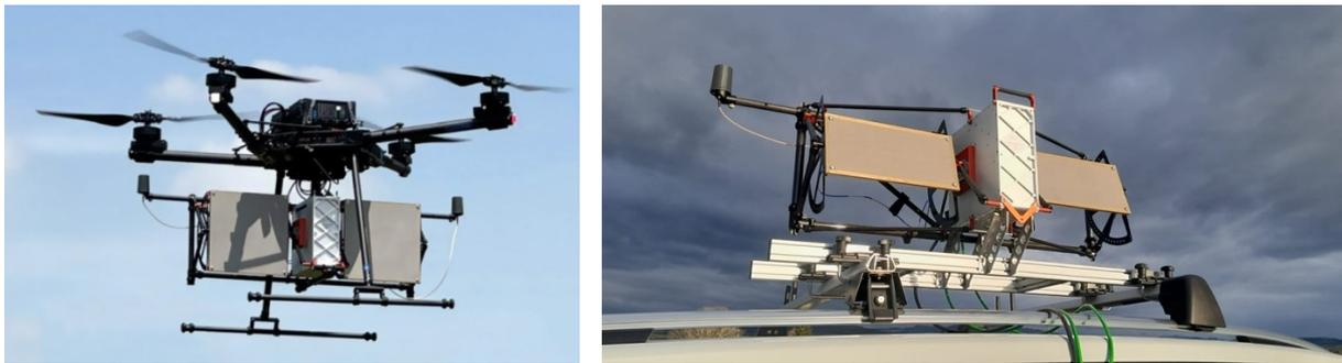
*Figure 1: Gamma L-Band SAR with carbon frame, patch antennas, and integrated GNSS/INS navigation system mounted on a Freefly Alta X quadcopter UAV (left) and a Gamma S-Band SAR mounted on a car roof rack (right) for repeat-pass interferometric SAR acquisitions in single-, dual-, or quad-polarimetric acquisition mode.*
