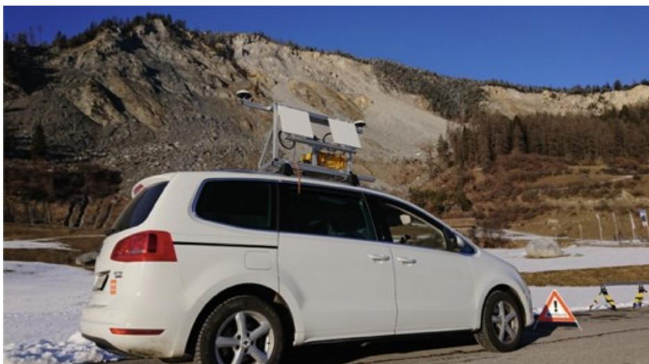
Figure 8: Car-borne Gamma L-band SAR setup with Honeywell HGuide n580 GNSS/INS system at the Brinzauls landslide.
