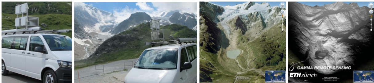
Figure 6: Left/center-left: car-borne setup of the L-band SAR system with one transmit and three receive antennas. Repeated SAR data acquisitions of the Stein Glacier were made while driving on a slightly curved section of mountain road. Center-right/right: Google Earth view of the Stein Glacier test site (CH). Geocoded intensity image (right) overlaid to Google Earth view as obtained from a car-borne L-band SAR acquisition.
